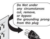
Power supply cord with 3-prong grounding plug
